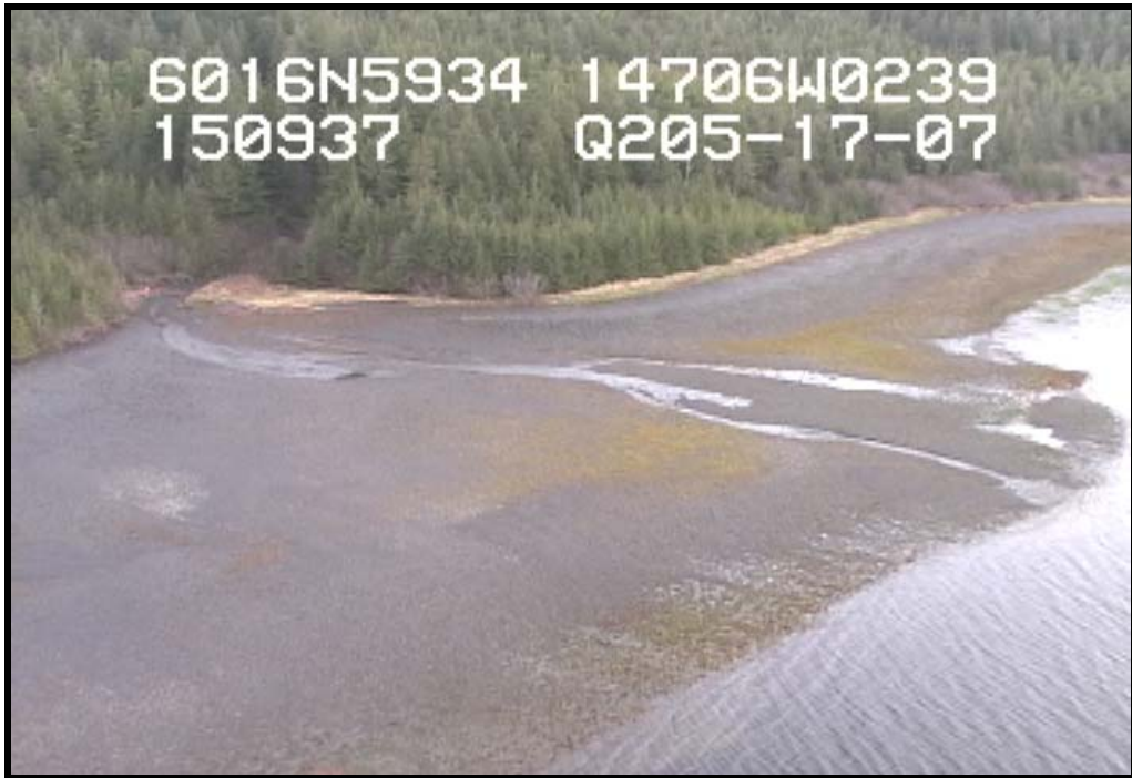
Figure 2. Example of a frame capture from video imagery in Zaikof Bay, northern Montague Island, Prince William Sound. Note GPS location, time code, and date burned on imagery, information which is also recorded in the navigational trackline.
